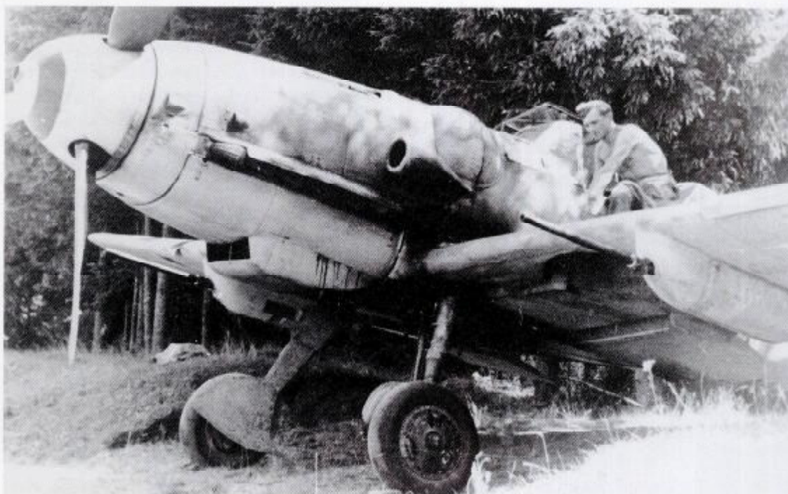
LEFT: In order to knock down four-engined bombers, the weight of German fighter armament was increased, as shown on this Bf 109 G-6 with 20 mm MG 151 cannon in the underwing gondolas. However, as this placed German single-engined fighters at a severe disadvantage when engaged by Allied escort fighters, the Luftwaffe introduced the concept of engaging the bombers with heavily armed Sturmgruppe protected by an escort of lightly armed fighters.
