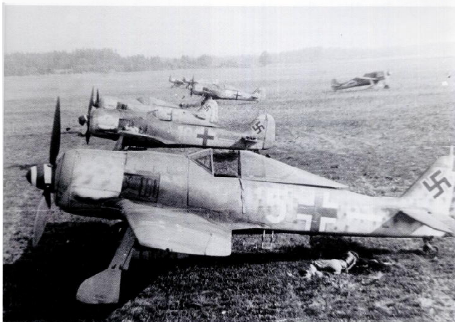
ABOVE: Aircraft of II./JG 300 at Holtzkirchen at the end of August 1944. In the foreground is an Fw 190 A-8/R2 of 7./JG 300, W.Nr. 681366, which was later shot down on 11 September. Note the external armour plate added to the sides of the windscreen and the sides of the cockpit. The fuselage armament has been deleted to offset the increased weight of the armour and improve manoeuvrability.
