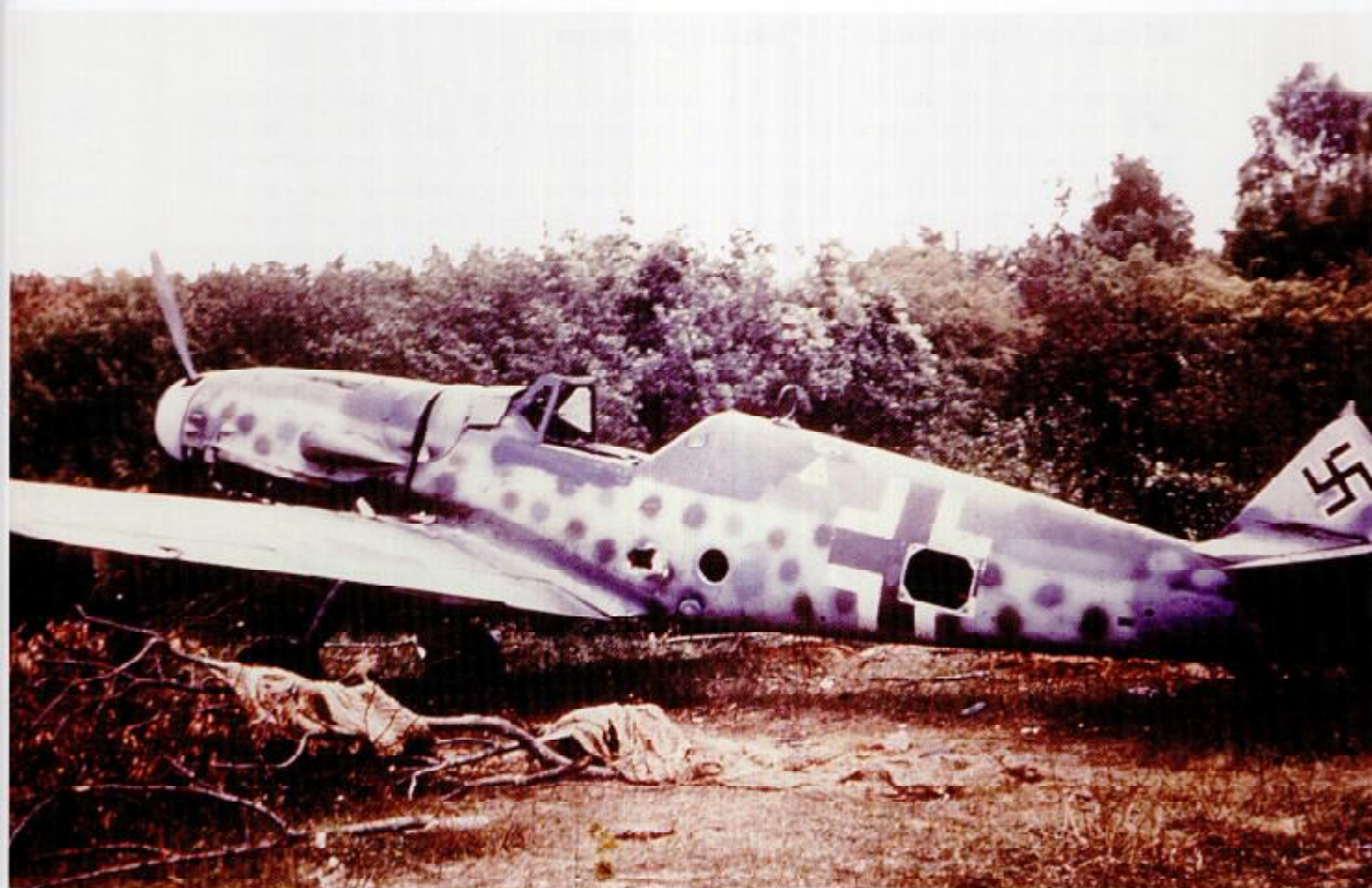
ABOVE AND RIGHT: The appearance of this Bf 109 G found at Rheims is typical of the finish applied to Bf 109s in 1944, although in this instance the machine has no operational markings. The camouflage scheme consists of the colours 74, 75 and 76 with regular, round mottles on the fuselage sides and, also typical of the period, is the grey centre to the fuselage cross which contrasts with the black of the swastika on the fin. Less typical, however, is the spinner, which has the appearance of being white with a black spiral, instead of the opposite way around.
