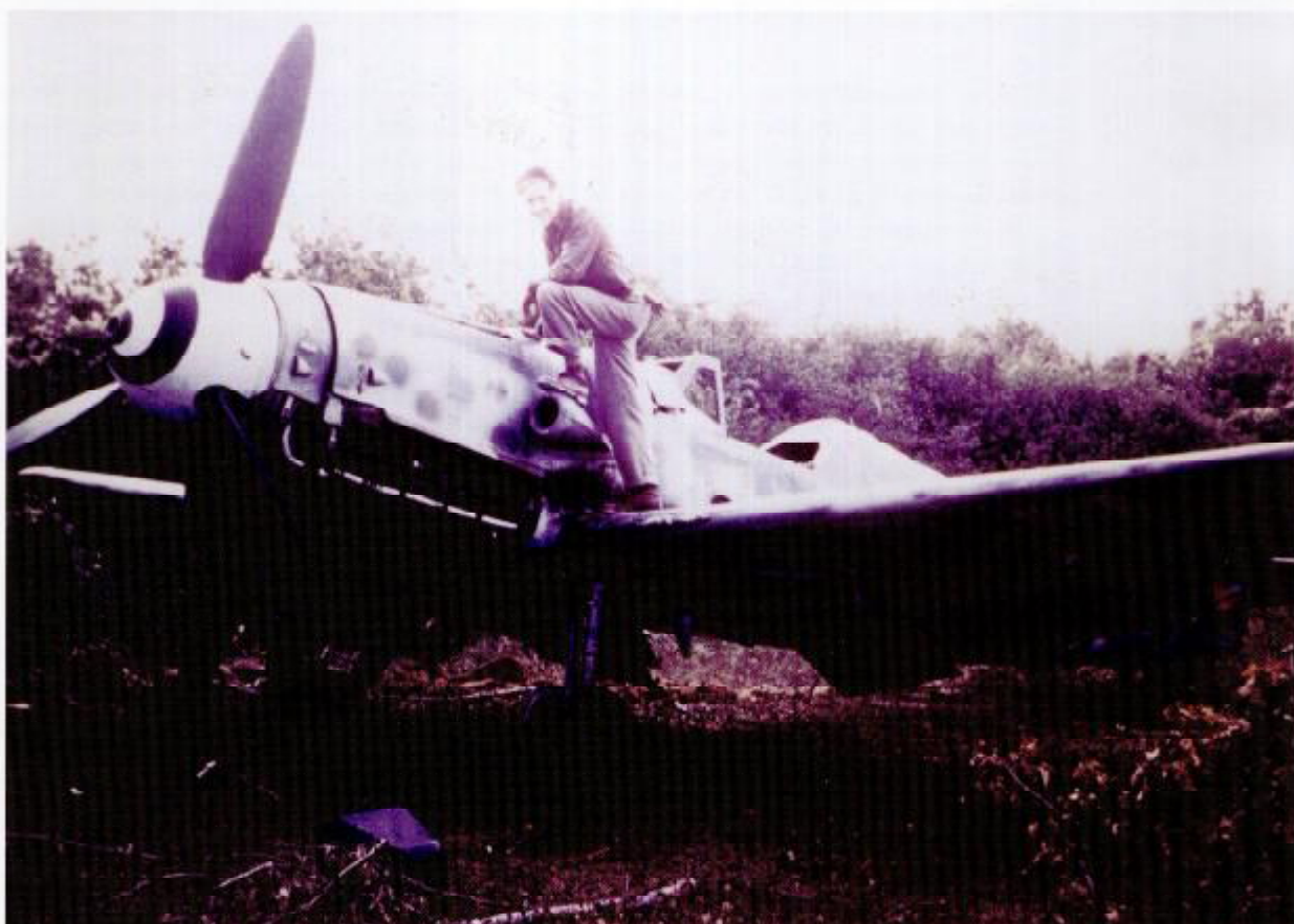
ABOVE AND RIGHT: The appearance of this Bf 109 G found at Rheims is typical of the finish applied to Bf 109s in 1944, although in this instance the machine has no operational markings. The camouflage scheme consists of the colours 74, 75 and 76 with regular, round mottles on the fuselage sides and, also typical of the period, is the grey centre to the fuselage cross which contrasts with the black of the swastika on the fin. Less typical, however, is the spinner, which has the appearance of being white with a black spiral, instead of the opposite way around.
